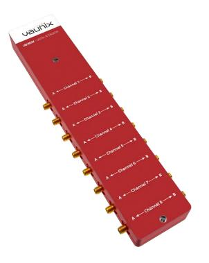
The Lab Brick LDA series of Digital Attenuators bring affordability, functionality, reliability and simplicity to the microwave test bench. The LDA products range from 6 MHz to 40 GHz with input level tolerance to 2 Watts and step size as small as 0.1 dB.
