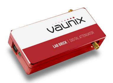
The Lab Brick LDA series of Digital Attenuators bring affordability, functionality, reliability and simplicity to the microwave test bench. The LDA products range from 6 MHz to 20 GHz with input level tolerance to 2 Watts and step size as small as 0.1 dB.
