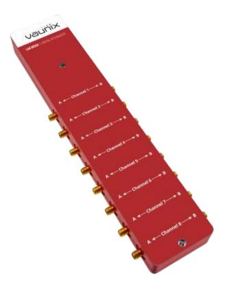
The Lab Brick LDA series of Digital Attenuators bring affordability, functionality, reliability and simplicity to the microwave test bench. The LDA products range from 6 MHz to 20 GHz with input level tolerance to 2 Watts and step size as small as 0.1 dB.
